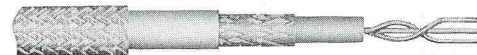
Armored Jacket over Single Shield—Solid Center Conductor Supported in Hollow Polyethylene Tube by Twisted Polyethylene Threads
